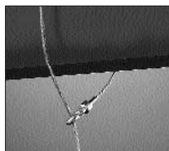
2. Connect hook to wire rope
